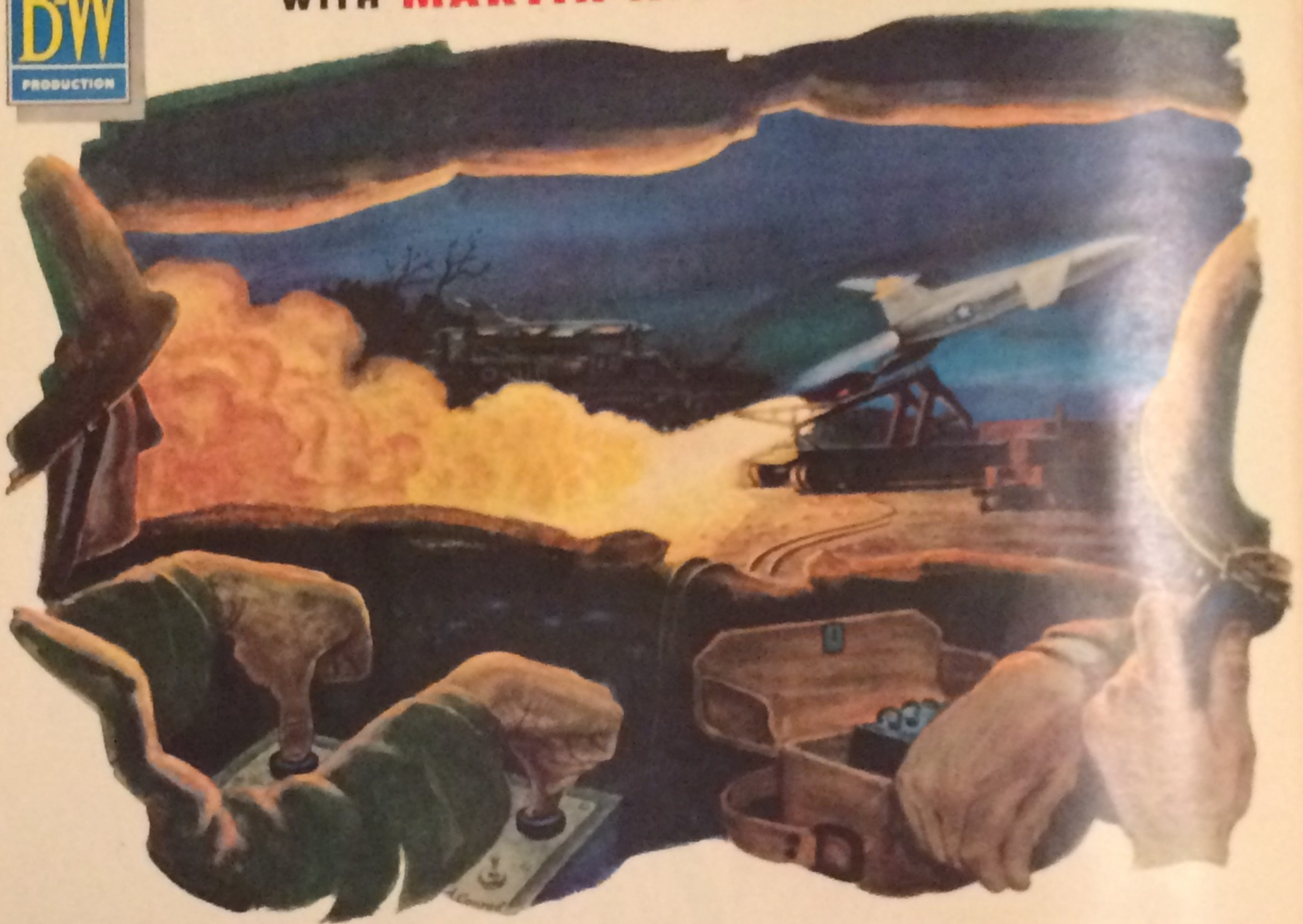
...3...2...1...FIRE! The Martin Matador B-61 pilotless bomber is launched in a fury of flames, its jet engine aided at take-off by a rocket.
