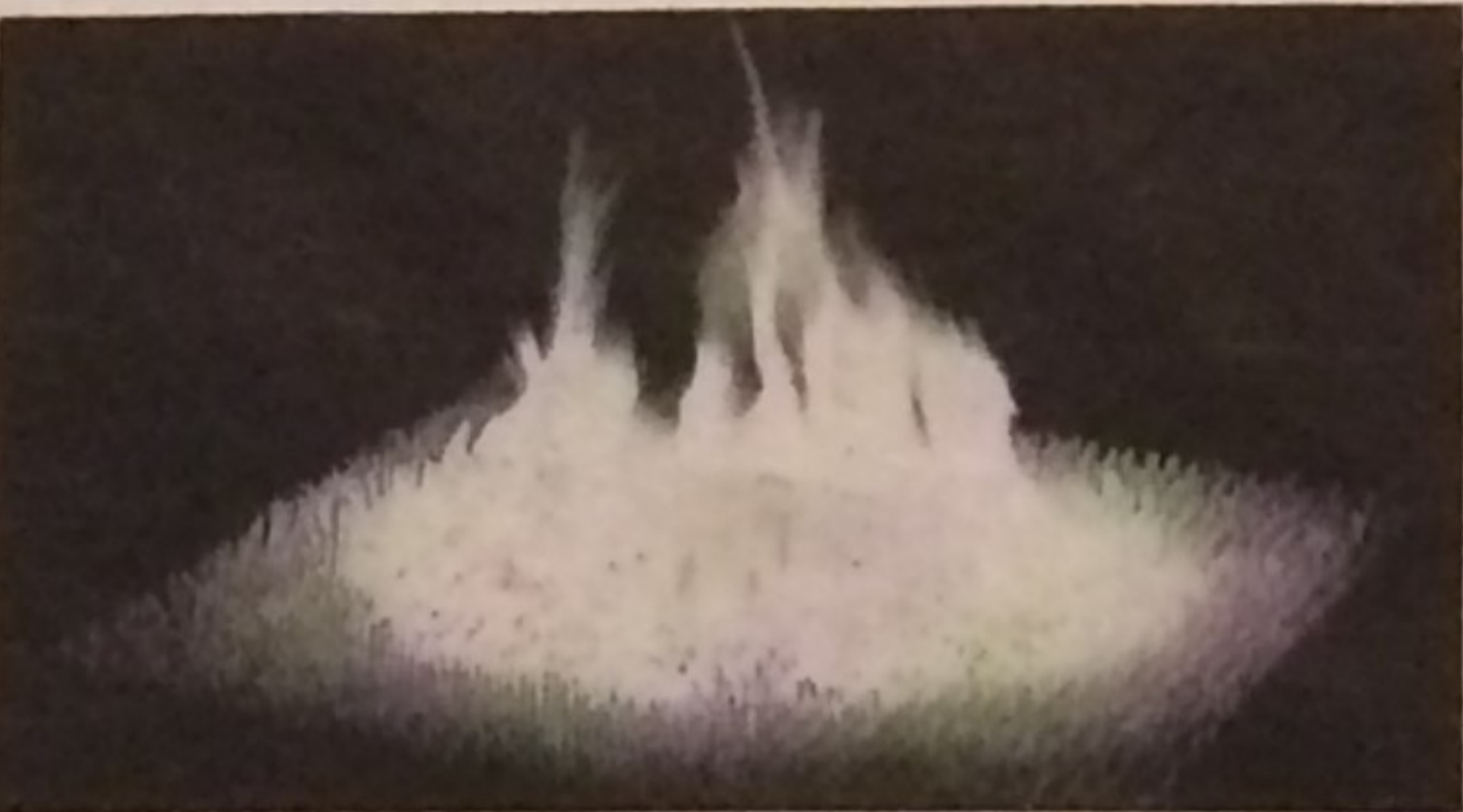
DEMONSTRATION OF FIRE STORM, which might follow an H-bomb explosion, was worked out by Engineer Ralph Healey of the New York Telephone Co. using 2,000 candles. Fires started by bomb (top left) would heat air
