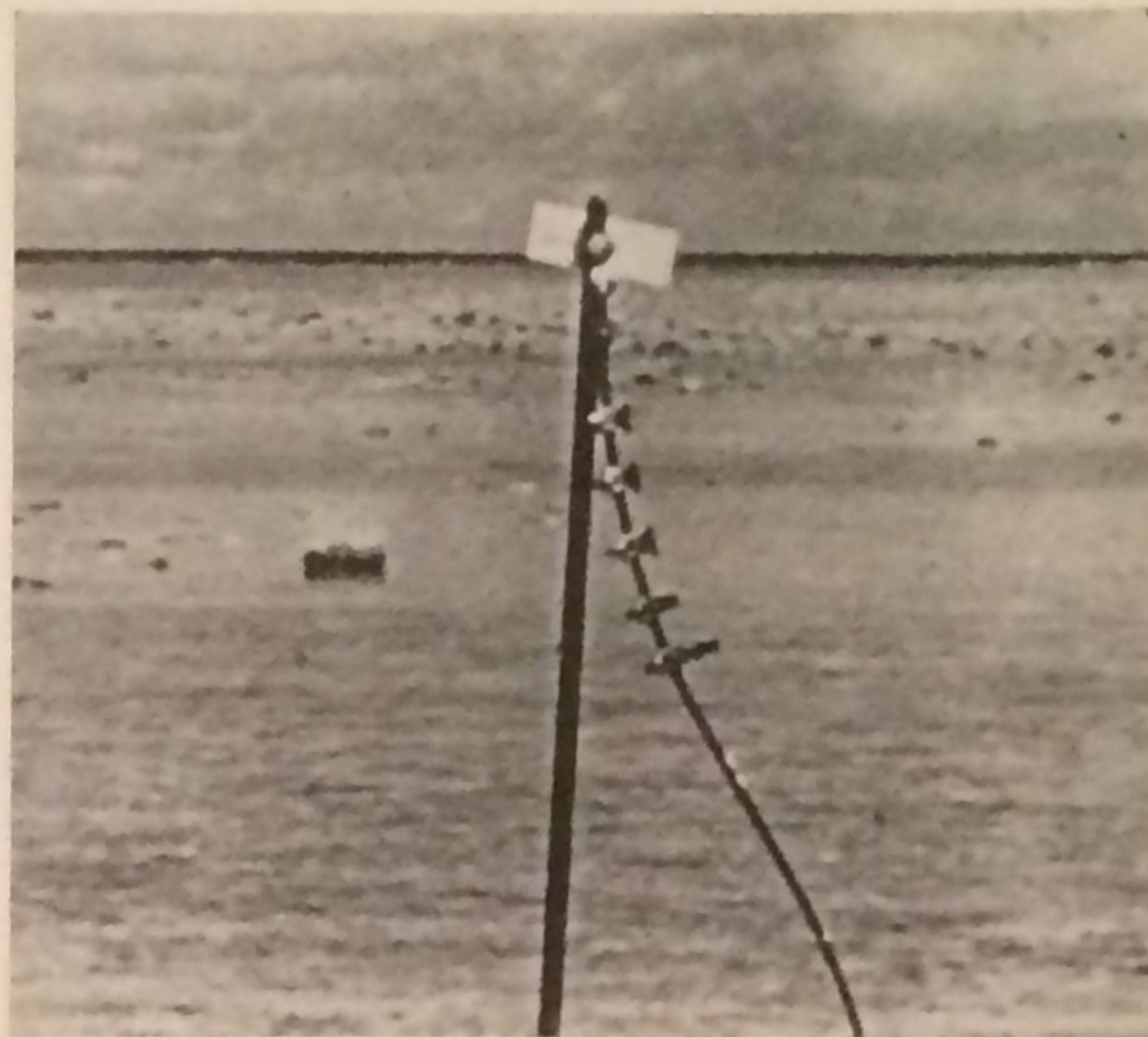
INSTRUMENT POST , one of a series located at different distances from Elugelab Island, may have recorded energy of weapon's neutrons or its X-rays.
